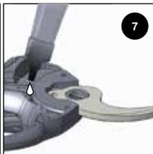
Clean and grease all parts including the pinion.
