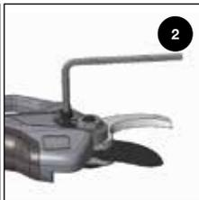
Turn the tool around and unscrew the center bolt lock.
