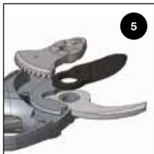
Take out and separate the driving system and the blade.
