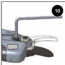
Tighten the center bolt lock.
