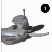
Remove the cover of the blade driving system.
