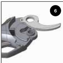
Remove the counter blade if it is necessary to change it.
