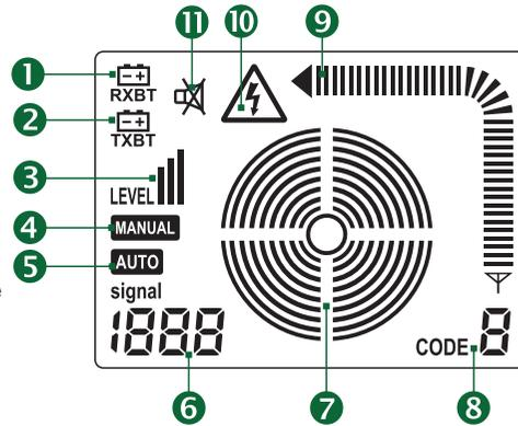
◆ 1.3.5 Display of receiver under cable locating mode
