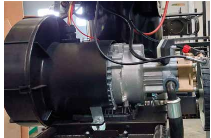
D125 PT'03 Motorpump with bigger brass head, double rubber sealing system (longer life)
