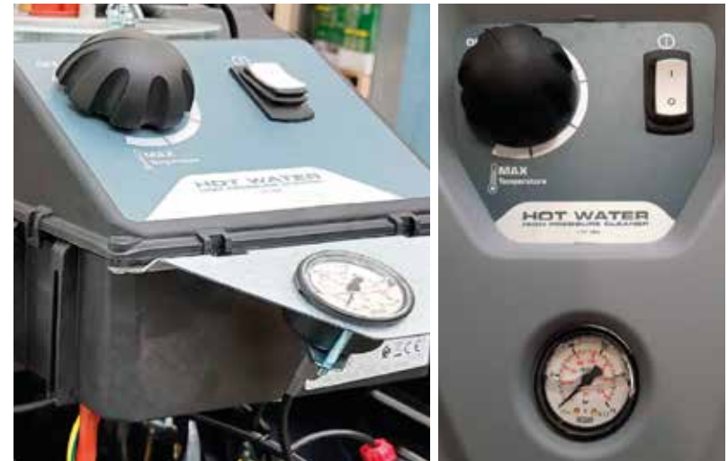
Larger DN50 pressure gauge mounted on a metal support on an upper control panel, flexible pipe for pressure signal
