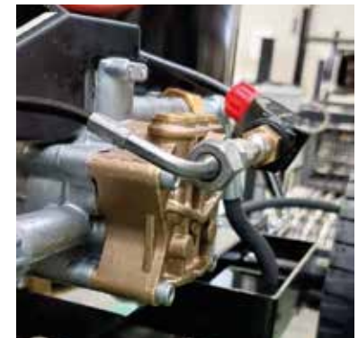
D125 PT'03 Motorpump with bigger brass head, double rubber sealing system (longer life)
