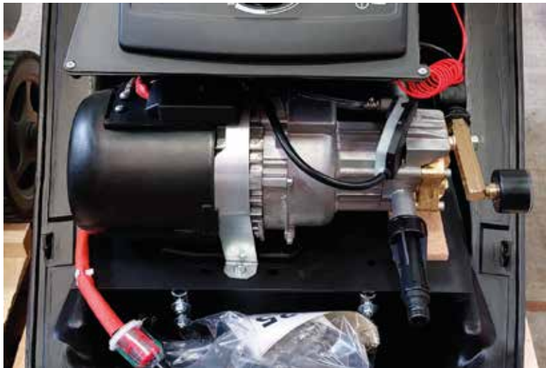
D125 PT'03 Motorpump with brass head and simple rubber sealing system
