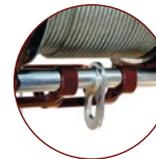
**6** The Pulley Hook allows double lifting capacity.
