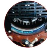
**8** New designed bearing system allows free rotating of the cable drum and increases the lifetime of the hoist.
