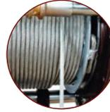
**5** Easily change the steel rope without needing to disassemble.
