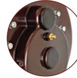
**9** Easily lubricate via the grease nipple.
