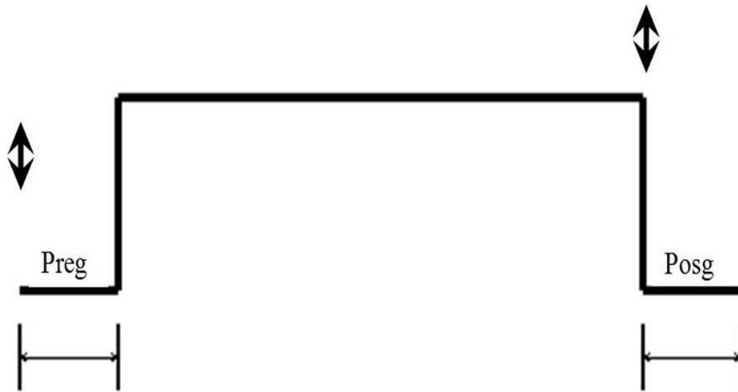
Pic14. 4T Operation
