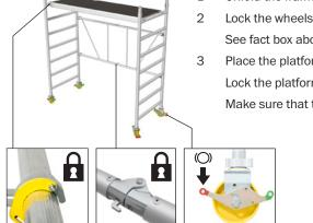
See fact box about wheels page 6. Place the platform on the desired height. Lock the platform locks. Make sure that the scaffolding does not lean but is standing straight.
