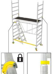
4 If you are building XR-scaffolding; Attach a base-ladder under the hatch of the platform (In Sweden the base-ladder can be excluded if the highest platform of the scaffolding is not placed higher than 2,5 meters).
